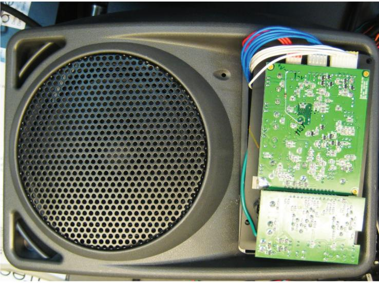
2. Invert Preamp so that rear of PCB is exposed
